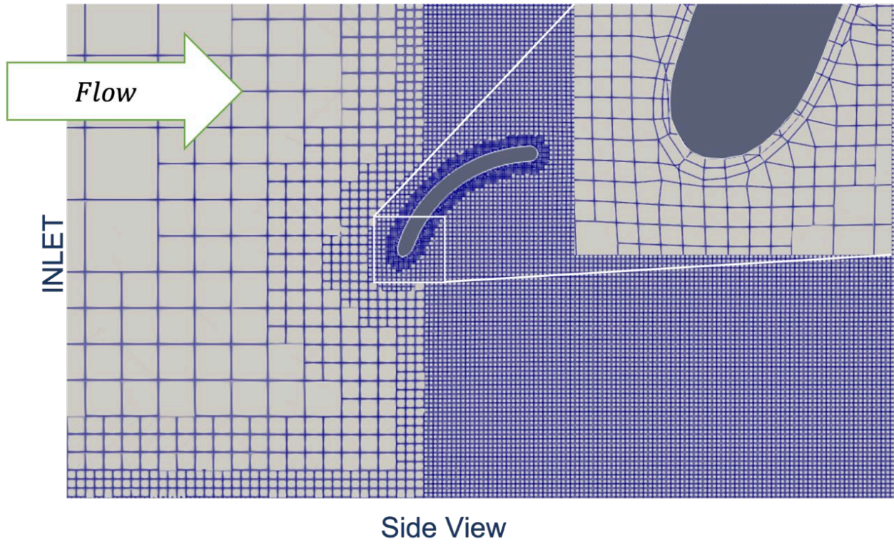
Figure 1. The cross-sectional area of the meshed domain around a rotated shell fragment shape with an aspect ratio of 1 and a flatness parameter of 0.2. The fragment is centered within the hydrodynamic boundary at a distance 15 cm away from the inlet and 6 cm from the bottom surface. Refinement zones in the wake and bottom wall surfaces increase the resolution to 0.7 mm and 0.3 mm, respectively. The resolution of the wall boundary layers at the shell fragment surface is 0.059 mm, corresponding to y^+ of order 1, fully resolving the viscous sublayer. Resolving the wall boundary layer allows us to forgo the use of wall functions, resulting in a more accurate measure of the surface forces experienced by the shell fragment.
